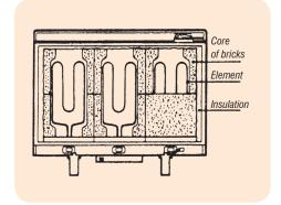
At the top of the box is a damper flap which can be opened to let the heat out. The more this flap is opened, the faster heat can escape from the heater into the room.
